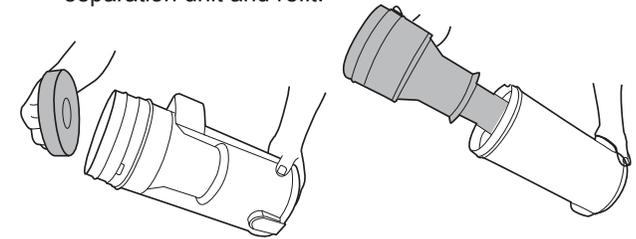
**4** Wash both filter and sponge under warm water until the water runs clean. Remove excess water by shaking and leave to dry for 24 hours. Reassemble and refit filters to cleaner, only when they are completely dry.
