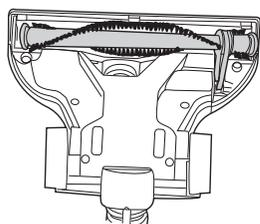
**NOTE:** When the brush was blocked and stopped rotating, switch off and remove the plug from the electricity supply, then use a pair of scissors to cut through any threads or hairs caught around the brush. Reassemble the brush and brush guard.
