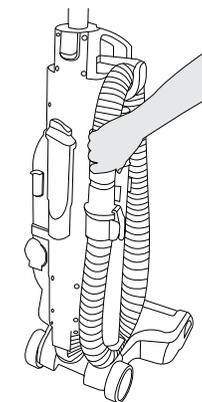
Removing a blockage from the mini turbo nozzle. Open the nozzle at each side, lift cover and remove the blockage.
