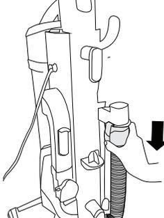
3 Plug the lower hose end in the hose socket.
