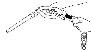
The hose can be removed at both ends.
