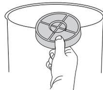
**2** Take out the pre motor filter and the separation unit from the dust bin. Clean excess debris from the separation unit and refit.
