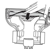
Check for a blockage in the hose socket. Use a flexible rod to remove any obstruction.
