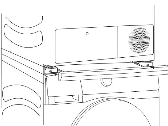
5. Install the left and right fixing clips on the left and right supports respectively as shown in the figure, and then fix them with 2 round head screws.
