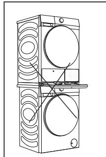
⚠ Bearing capacity exceeding 18 KG is not allowed for the support.
