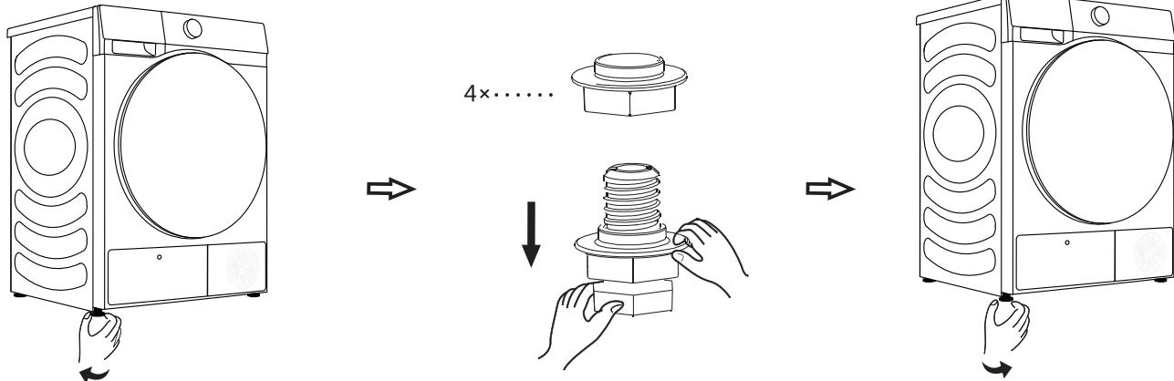
2. Unscrew the 4 feet of the clothes dryer, insert the 4 foot accessories into the feet as shown in the figure, and then reinstall the feet in place.
