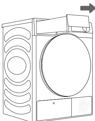
3. Draw the water box, and empty it if there is residual condensate water in it. (This step can be ignored for new machines)
