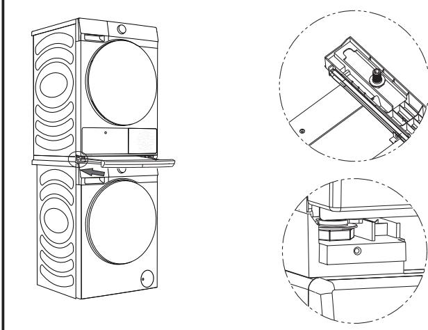
4. Take out the drawer board and place dryer on the rail of supporting bracket. Make sure that 2 feet at the back are placed according to the diagram, then push in direction of the arrow. Finally put all 4 feet in the socket of the bracket based on the diagram.
