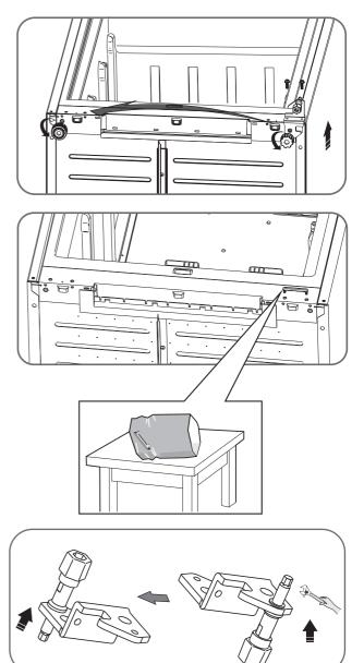
8. Replace the lower hinge part to the left side and fixing it with the special flange screws. Replace the adjustable bottom feet part to another side and fixing it.
