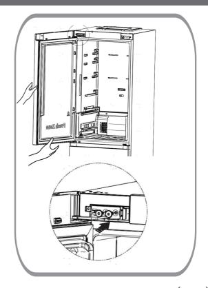
11.Reinstall the door corner cover(right), the door corner cover(left), the case corner cover(right) and the case corner cover(left) which are taken from the accessory bag.
