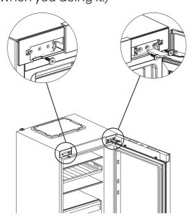
3.Remove the door and place it on a smooth surface with its panel upwards.Loose 2 self-tapping screws, detach the stopper,the door backstop and the shaft sleeve, then install the stopper, the door backstop and the shaft sleeve to the left side with 2 self-tapping
