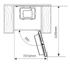
The total space required for the refrigerator to fully open the door in the built-in status
