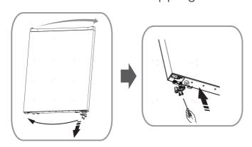
6. Change screw hole covers on middle cover plate from left to right (as shown in figure below).
