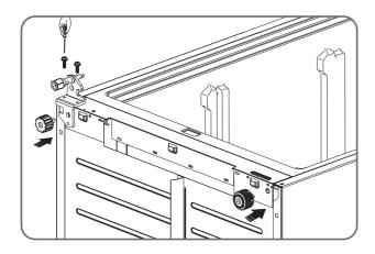
9. Move the lower door and adjust position to align lower hole site and lower hinge axis. Turn the middle hinge by 180°, adjust the middle hinge to the appropriate position and then install it.
