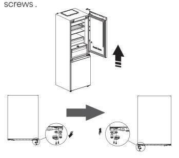
4.Loose screws used to fix the middle hinge and remove middle hinge part. Then remove the lower door.
