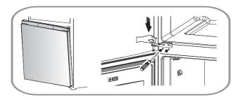
10.Transfer the upper door to appropriate position. Align the lower hole of the upper door with the upper hinge shaft of the middle hinge, then align the upper hole of the upper door with the hinge shaft of the left upper hinge. Finally adjust the left upper hinge to the appropriate position and then install it with 2 screws.
