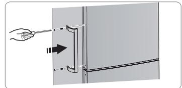
3. Fix the handle with the special screws provided in the plastic bag, then install the handle covers.
