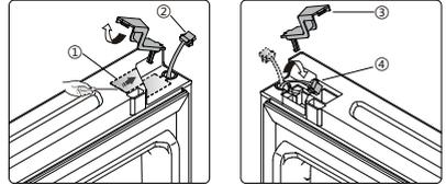
8. Loose screw ③ and take down part ② and part ①, Install replacement door stopper-left ④ and stop block-left ⑤ (provided in the plastic bag) to the left side with screw ③. Keep part ① and part ② with the appliance for future reference.
