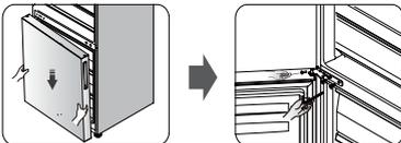
16. Transfer the upper door to the appropriate position. Secure the door level, make the middle hinge axis into the lower hole of the upper door. Install the hinge② (provided in the plastic bag) by screws①. Please hold the upper door by hand when installing.
