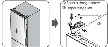
17. Take out the connector② and③ from the top left side. Connect① with②, then connect③ with the door switch on the upper hinge cover-left.
