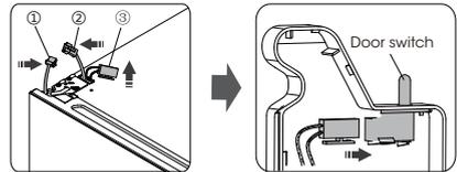
18. Install the upper hinge cover② on the left corner by screw①.
