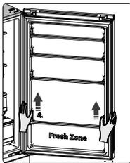
6. Install cover ① (provide in the plastic bag) on the top right side. Then remove cover ② from top left side of the appliance, and put it into the plastic bag.
