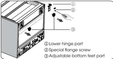
13. Loosen the lower hinge pin, change it to the reverse hole site, then tighten it into position follow the picture below.
