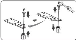
14. Replace the lower hinge part to the left side and fixing it with the special flange screws. Replace the adjustable bottom feet parts to another side and fixing it.
