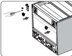
15. Stand the refrigerator upright and carefully slot the lower door onto the lower hinge pin and hold in position. Install middle hinge-left (in the plastic bag) ensuring the lower door is secured in place.
