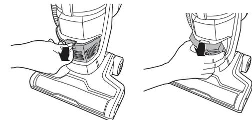
**2** Remove the exhaust filter by pressing the latch on both sides.
