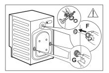
7. Close the holes with the plastic caps you find in the user manual bag. Put the smallest cap F in upper hole and the two bigger caps G in lower holes.
