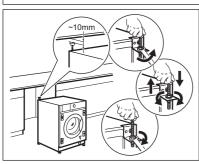
2. Adjust the anti-tilting device so that the distance from the counter is 10mm. Loosen the nut counterclockwise with a 3mm wrench. Adjust the height and turn the nut clockwise to fix it.
