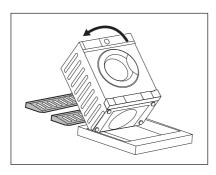
**1.** Put two polystyrene packaging elements on the floor under the appliance.
