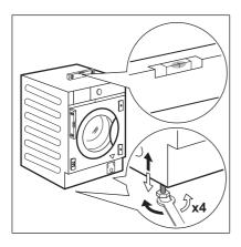
thick, under the appliance. It should be screwed to at least 2 floor beams and should extend beyond the front feet.
