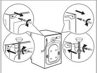
1. Remove the screws of the top cover on the rear of the appliance and install the anti-tilting device as shown in the drawing.
