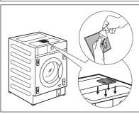
The appliance is also equipped with an adhesive sponge pad H that you can find inside the drum. Attach it on the top of the appliance where indicated in the drawing.
