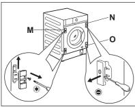
If the cupboard door has to be opened from left to right, invert the position of the hinge supports  ${\bf M}$  with the magnetic plate  ${\bf N}$  and lower plate  ${\bf O}$ .
