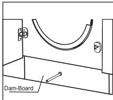
2. Turn the filter down as shown with the figure and take out sundries matters.
