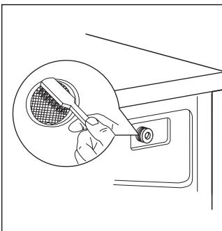
5. Reinstall the filter to the water inlet and reconnect the water supply hose.
