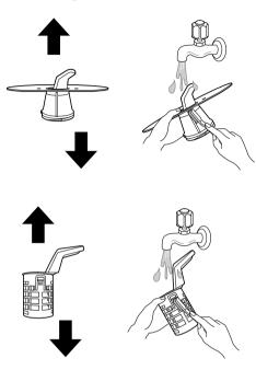
4 To replace the assembled filters, position the spray arm so the wider vee is toward the front. Fit the filters back into the filter holder and secure them by turning the inner filter clockwise until it clicks into place.
