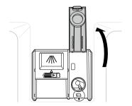
Add a liquid rinse aid to the maximum fill level. The rinse aid should be settled in the dispenser while filling, or air bubbles may result in poor drying results.
