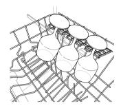
The right side row of tines can be folded down or the cup racks can be folded up out of the way for tall crockery items.
