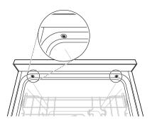
Pull the top cover backwards after removing the two screws and then lift it up to remove it.
