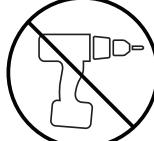
• We do not recommend the use of power drill/drivers for inserting screws as this could damage the unit. Only use hand screwdrivers.
