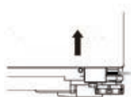
Insert the "C" type gasket
