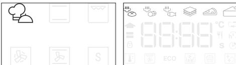
Turn the rotary knob to select from amongst the subfunctions available on the right-hand display and then press to confirm.
