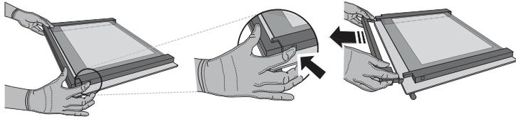
2. Lift and firmly hold the inner glass with both hands, remove it and place it on a soft surface before cleaning it.
