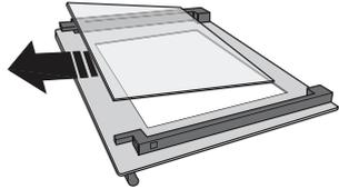
3. Refit the intermediate pane (marked with "1R") before refitting the inside pane: To position the panes of glass correctly, make sure that the "R" mark can be seen in the left-hand corner. First insert the long side of the glass marked "R" into the support seats, then lower it into position. Repeat this procedure for both panes of glass.
