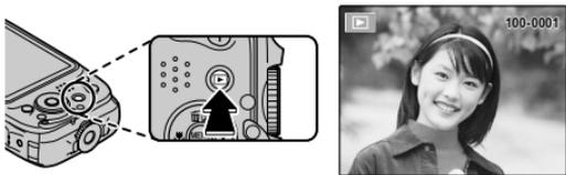
Press the selector right to view pictures in the order recorded, left to view pictures in reverse order. Keep the selector pressed to scroll rapidly to the desired frame.
