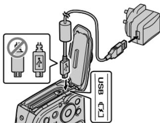
Connect to camera Micro USB connector (Micro-B)
