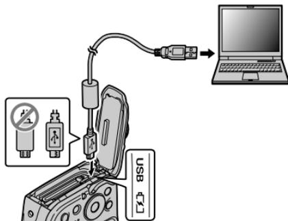
Connect to camera Micro USB connector (Micro-B)
