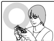
To prevent pictures that are out of focus or too dark (underexposed), keep your fingers and other objects away from the flash and from the protective glass covering the lens.
