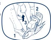
6. Push the choke control (A) in to disengage. (Failure to do this may cause the engine to flood).
