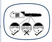
**CAUTION!** If the saw chain is TOO LOOSE or TOO TIGHT the clutch, chain bar, chain and crank shaft bearing will suffer premature wear. Above fig. shows the correct tension A (when cold) and tension B (when warm). FIG C shows a chain that is too loose.
