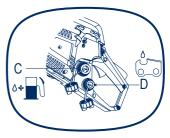
Clean surface around fuel cap to prevent contamination. Loosen fuel cap slowly. Rest the cap on a clean surface. Carefully pour fuel into the tank. Avoid spillage. Prior to fastening the fuel cap, clean and inspect the seal located inside the fuel cap. Immediately replace fuel cap and hand tighten. Wipe up any fuel spillage.
