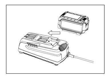
Mount the battery pack onto the charge by sliding into the guide rails.
