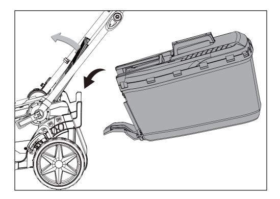
• Lift the deflector guard, then fit the grass bag onto the mounts at the rear of the mower, then release the deflector guard. Ensure the deflecto guard fits firmly onto the grass bag.
