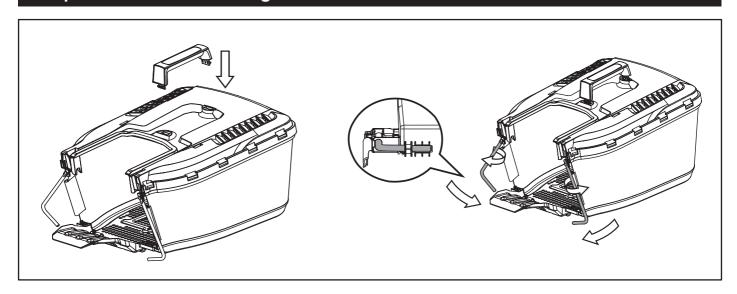
• Insert the collector handle into the grass bag upper, clip the plastic retainers onto the metal frame, and ensure the side clamping sleeves are properly fixed on the frame.
