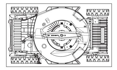
If the blade is blunt, it can be sharpened in a specialised workshop. If the blade is damaged or showing signs of imbalance, it must be replaced.
