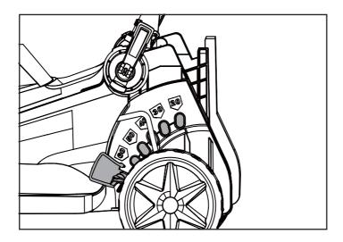
• To adjust the cutting height, gently pull the height adjustment lever towards you to disengage it from its existing position and move it to the desired cutting height position. Ensure it clicks back firmly into position.
