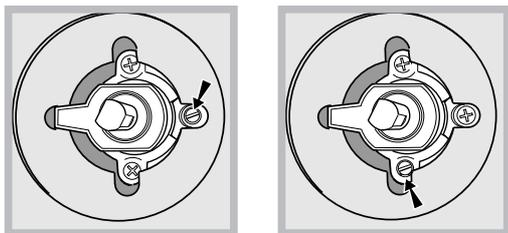
3. While the burner is alight, quickly change the position of the knob from minimum to maximum and vice versa several times, checking that the flame is not extinguished.
