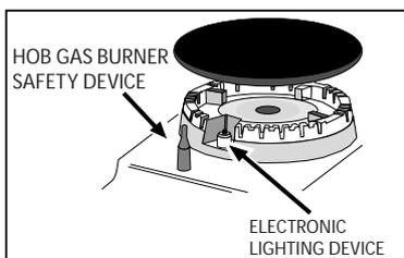
To switch the burner off, turn the knob until it reaches the stop position
