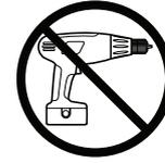
• We do not recommend the use of power drill/drivers **for inserting screws**, as this could damage the unit. Only use hand screwdrivers.
