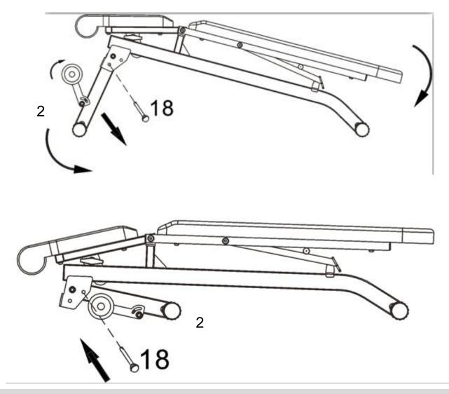
Remove the Lock Pin(18) and fold the Front Support Frame(2) and the Leg Developer(6). Then insert the Lock Pin(18) into the other hole to lock it in folding position as shown in the diagram.
