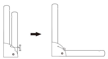
Slide the tube over the connector, depress the button continue to slide the tube until the button locates in the tube hole.
