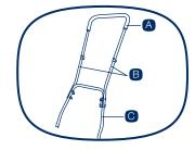
iii. Position the complete assembled handle over the studs of both sides on the rear of mower frame.
