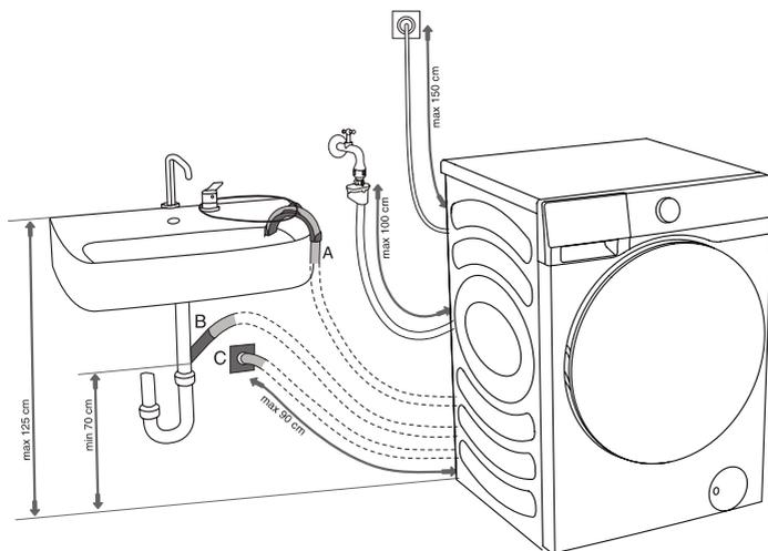
**A** Discharge hose end may be placed over a sink or a bathtub. B Use a string fed through the opening in the elbow support to attach the hose and prevent it from slipping to the floor.
