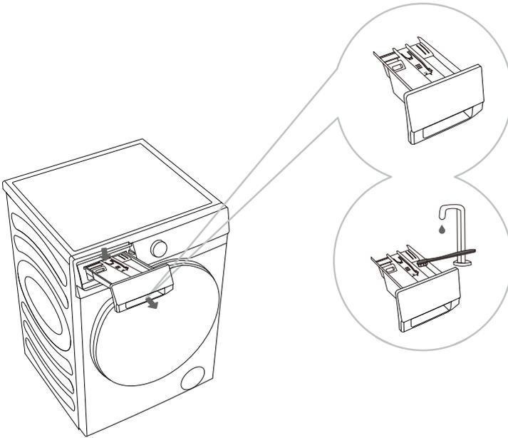
**1** To remove the detergent compartment from the housing, press the small tab.
