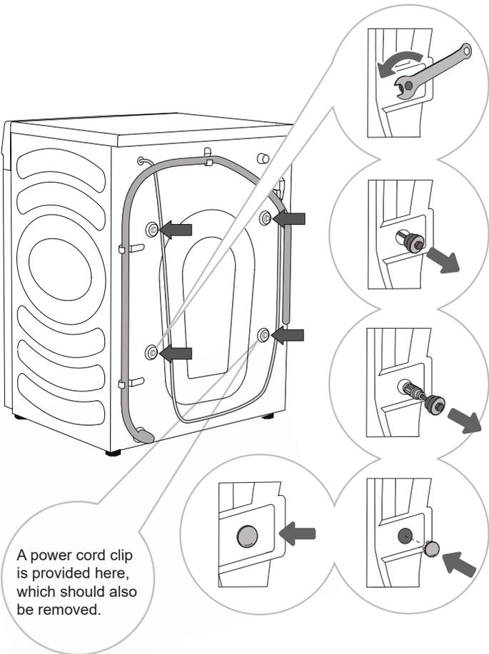
**1** Move aside the hoses and use a fitting spanner to undo the 4 screws on the back of the appliance by turning them counter clockwise, as indicated by the arrow. Undo them by approximately 30 mm (not completely).
