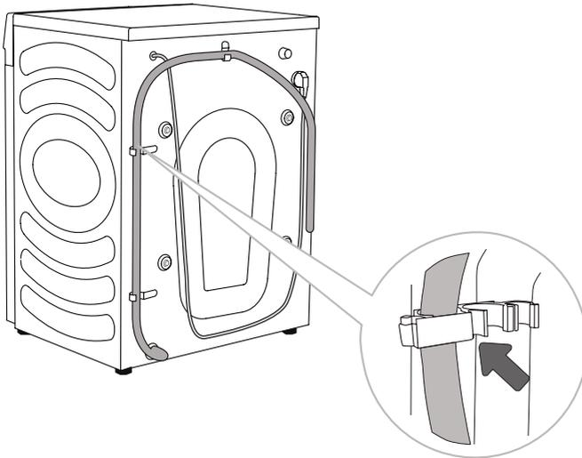
**D** The discharge hose has to be attached and affixed to the pin on the back of the washing machine, as shown in the figure.
