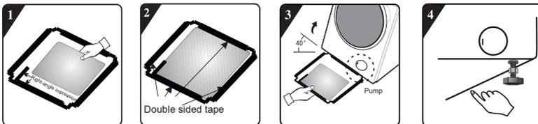
1. Before installing the noise reduction board, align and paste the acoustic absorption wool with and along the right-angle impression on the noise reduction board (this procedure is unnecessary for some of the models without acoustic absorption wool).
