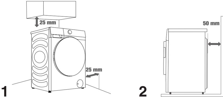
⚠ The washing machine may not be in contact with a wall or adjacent furniture. For optimum washing machine operation, we recommend observing the clearances from the walls as indicated in the figure.
