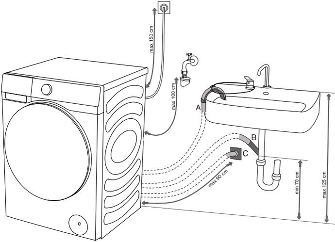
**C** Discharge hose can also be attached to a wall drain with a trap; such trap should be properly installed to allow cleaning.
