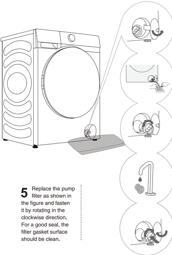
**5** Replace the pump filter as shown in the figure and fasten it by rotating in the clockwise direction. For a good seal, the filter gasket surface should be clean.
