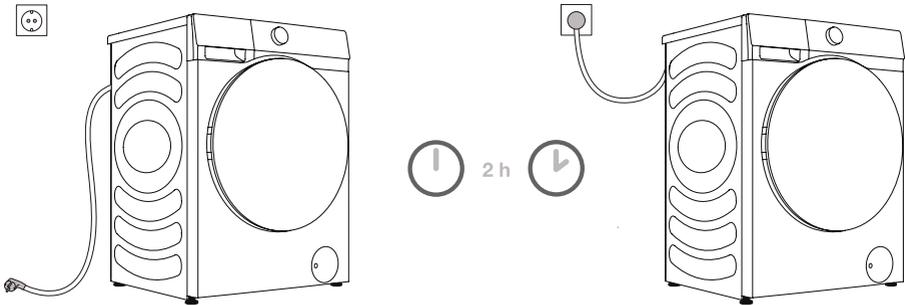
**⚠ Before connecting the washing machine to the power mains, wait for at least 2 hours until it reaches room temperature.**
