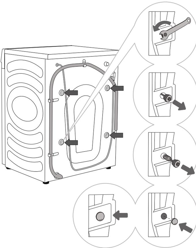
**1** Move aside the hoses and use a fitting spanner to undo the 4 screws on the back of the appliance by turning them counter clockwise, as indicated by the arrow. Undo them by approximately 30 mm (not completely).
