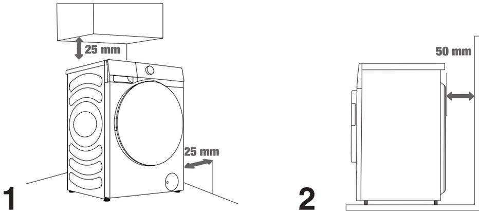
⚠ The washing machine may not be in contact with a wall or adjacent furniture. For optimum washing machine operation, we recommend observing the clearances from the walls as indicated in the figure.
