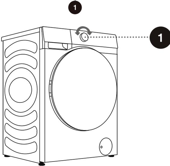
⚠ During operation, the programme selector knob (1) will not rotate automatically.
