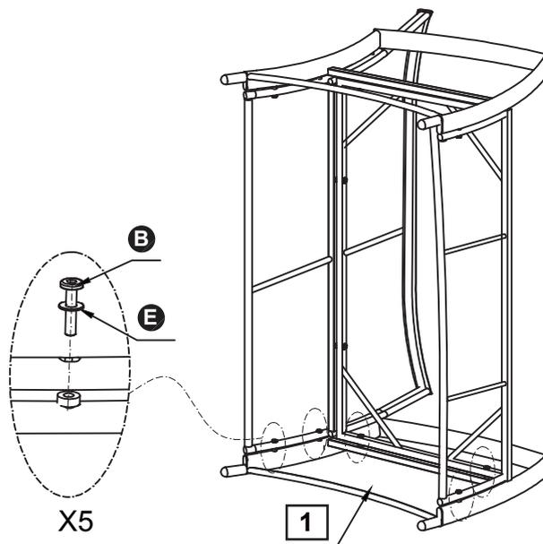
Tighten all the screws and cover all the screws with caps **F**.
