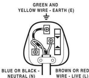
The BLUE wire must be connected to the terminal marked with the letter N p
