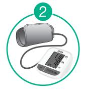
Plug the connector from cuff into the monitor on the left side.
