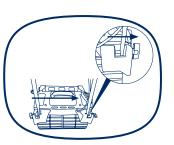
ii. Release the locking knobs and fold the handle down.
