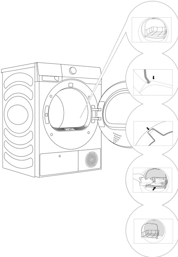
**1** Open the dryer door and insert the drying basket.
