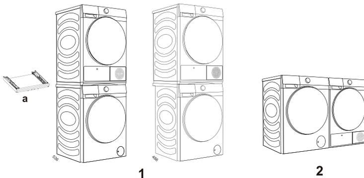
At least two persons are required to install the tumble dryer on top of a washing machine.
