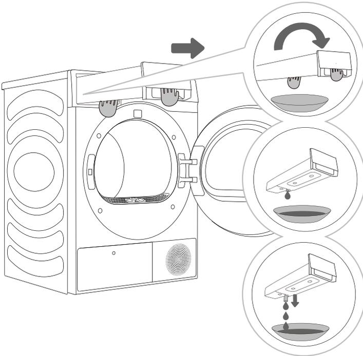
**1** Pull out the condensate tank from the dryer (using both hands as shown in the figure), then turn it upside down over a washbasin, sink, or any suitable vessel.
