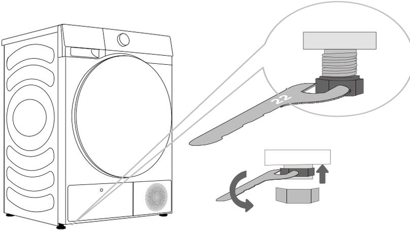
💡 Floor on which the dryer is placed must have a concrete base. It should be clean and dry; otherwise, the dryer may slide. Also clean the adjustable feet.
