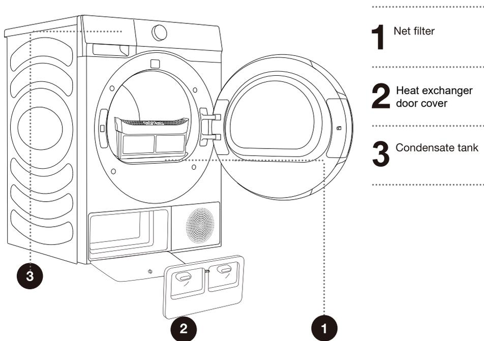
**⚠** The dryer may never be operated without the filters in place or with damaged filters, as excessive amount of accumulated fibres from the fabric could cause malfunction or failure of the dryer.
