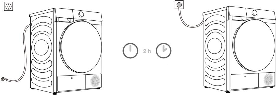
**⚠ After installation, the dryer should stand still for two hours before it is connected to the power mains; this allows the dryer to stabilize.**
