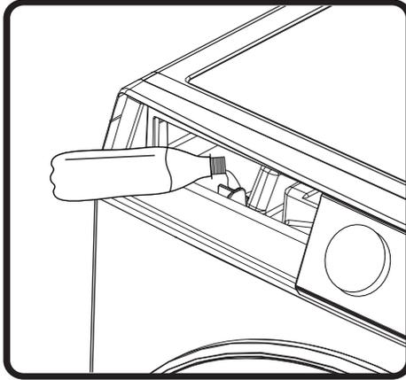
The water tank filter mesh could be blocked by impurities after long use; it is suggested to clean it on a monthly basis. Hold out your fingers to pinch and take out the lower water tank filter mesh; after washing the filter mesh, reinstall it properly.
