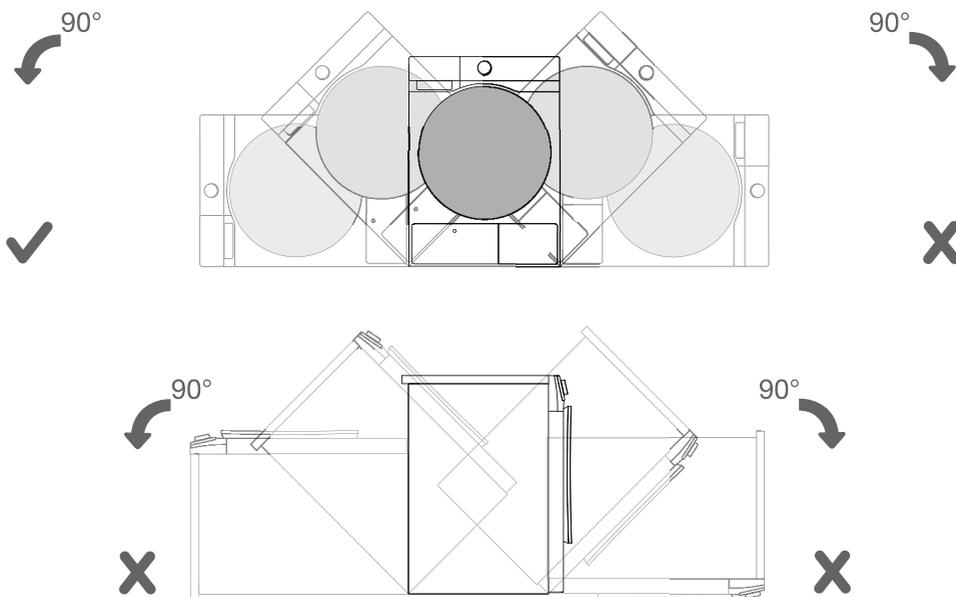
⚠ After installation, wait for 24 hours without moving the appliance before using it for the first time. If the dryer has to be laid down on one of the sides during transport or servicing, place it with its left side, viewing from the appliance front, downwards.
