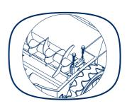
d. Slide the hex nut out the socket of driving shaft and the bearing from the support with the bolts and spring washers.
