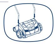
3. Secure the bars with one screw each to the support.
