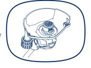
iv. Put the new spool in the spool housing, thread the line into the hole.
