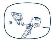
iii. Insert the bolt from the right through the opening. Ensure that the bolt head sits properly in the recessed shape in the support then tighten the knob.
