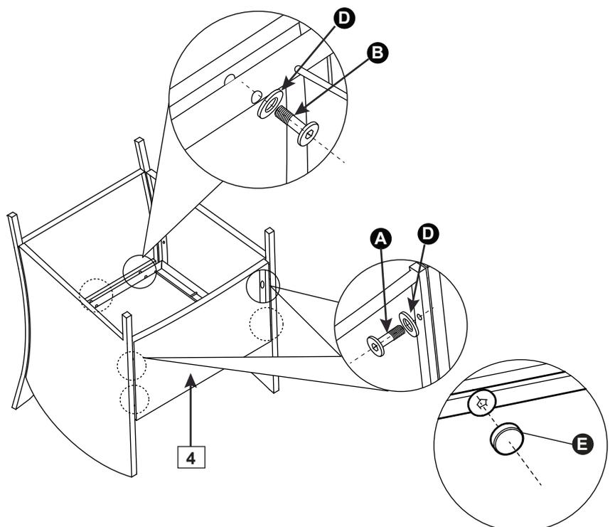
Tighten all the screws and cover all the screws **A** and **B** with cap **E**.
