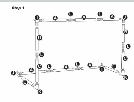
Join the tubes together with connectors as illustrated.
