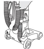
To clear a blockage in the Pet Hair & Allergen Remover\*, twist the collar at the rear and lift the cover.
