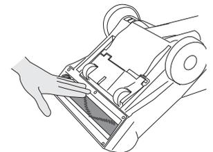
Check for a blockage in the hose socket. Use a flexible rod to remove any obstruction.
