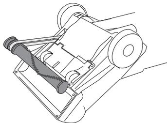
Loop the new belt around the motor and brush channel.
