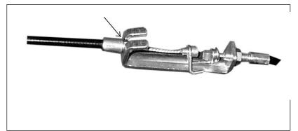
Drop down the Connector so the fitting sits firmly on top of the bracket.
