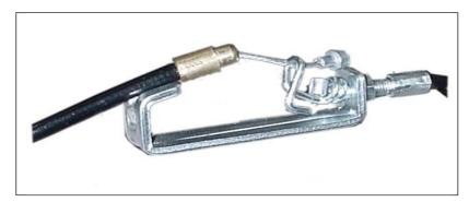
Slide the Cable wire from the extension sensor wire Connector in between the opening on the wire holder on sensor wire Connector.
