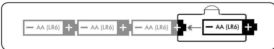
**Note:** You can check the base of your radio for the correct direction to install your AA Alkaline batteries.
