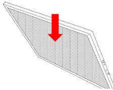
3. Clean the filter and allow to dry before replacing (refer to cleaning instructions on the following page).
