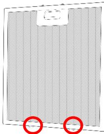
2. Press the lock in and push the filter upwards, locking it in place.
