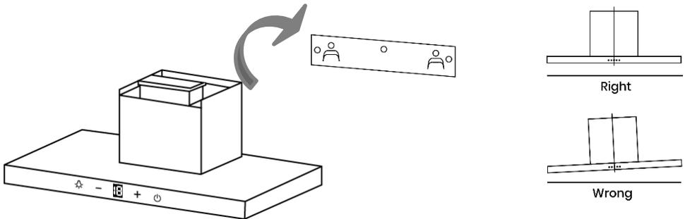
3. Remove the appliance from the hood fixing bracket and following installation, remove the film completely.
