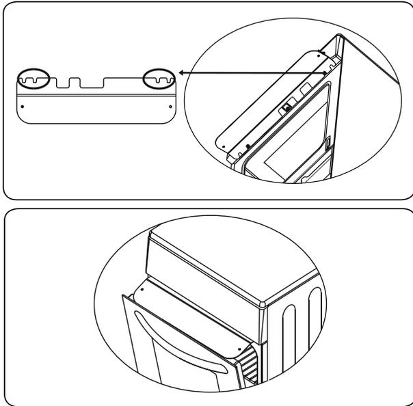
Hold the heat shield with the warnings facing upwards. There are two small slots on the right and left side of the rear edge of the shield, as shown in the figure.
