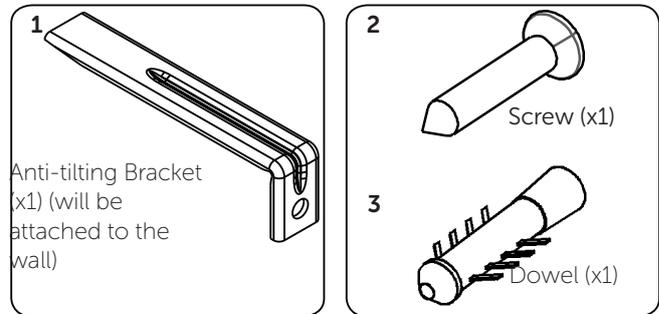
The document bag contains an anti-tilting kit. Loosely attach the anti-tilting bracket (1) to the wall using the screw (2) and dowel (3), following the measurements shown in the figure and table below. Adjust the height of the anti-tilting bracket so that it lines up with the slot on the cooker and tighten the screw. Push the appliance towards the wall making sure that the anti-tilting bracket is inserted into the slot on the rear of the appliance.
