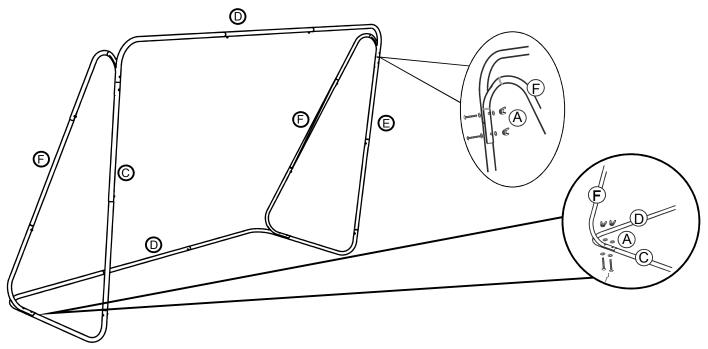
5. Drape the goal net (B) over the frame, make sure the red net tabs are top left and top right of the goal. The seam of the net should follow the frame supports. Secure the net to the frame using the net clip(N), ensure they are evenly spaced around the frame.
