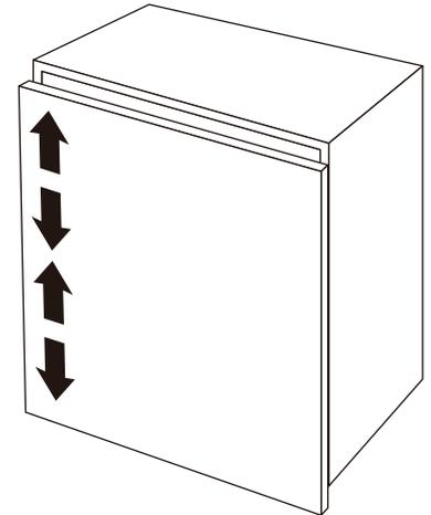
**b:** Try to work on the hinges one at a time. This will prevent the weight of the door pulling it out of position.
