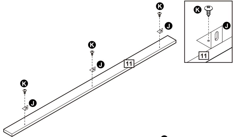
**b:** Use Screws **K** to fix the Front panel **11** onto the Bottom panel **2**.
