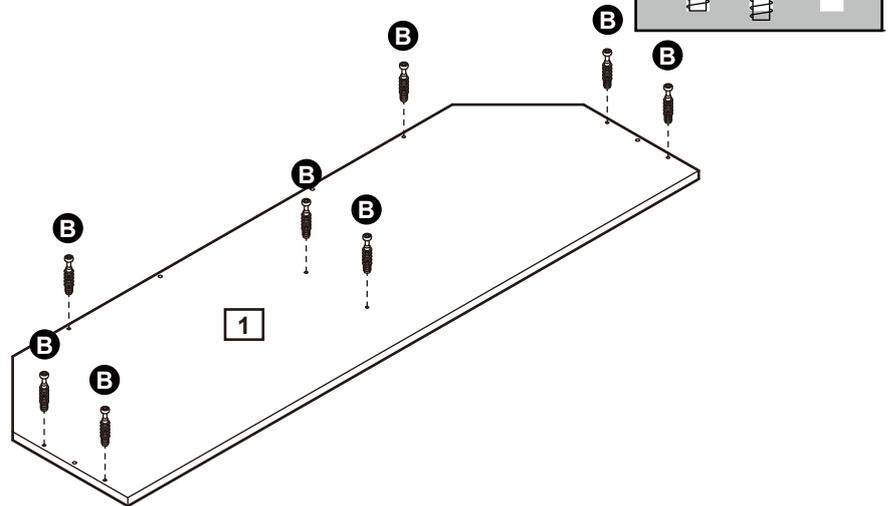
**b:** Carefully locate the Top panel **1** onto the unit.
