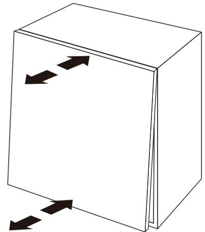
**c:** This method can also be used to straighten-up tilting or twisting doors.
