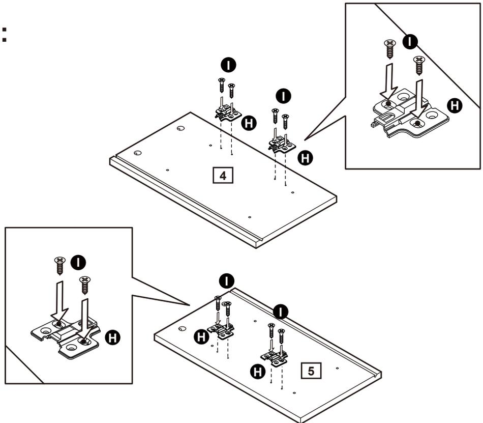
**b:** Screw Locking pins **B** into the Right side panel **4** and Left side panel **5**.
