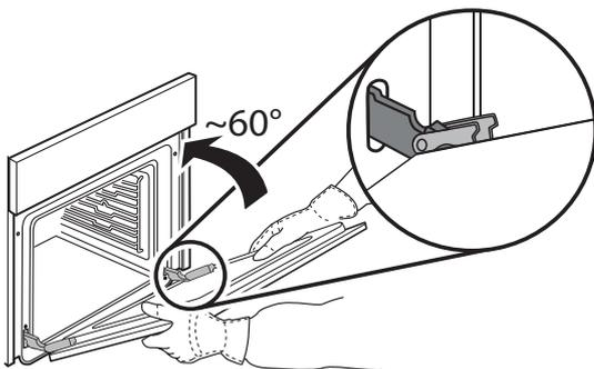
4. Take a firm hold of the door with both hands – do not hold it by the handle. Simply remove the door by continuing to close it while pulling it upwards at the same time until it is released from its seating.
