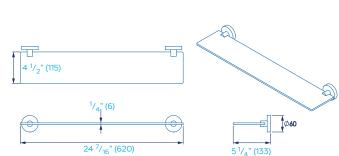
Dimensions:  $2\frac{1}{8}$  ×  $24\frac{7}{16}$  ×  $5\frac{1}{4}$  (H54mm × W620mm × D133mm)
