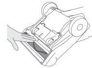
Refit the brush guard with 6 retaining screws.
