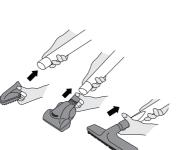
**IMPORTANT!** When using cleaning tools, the cleaner must be kept in the upright position, particularly when cleaning stairs. The nozzle height should also be set to tool mode.
