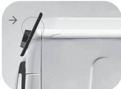
If you do not know the position of your NFC antenna, slightly move the smartphone in a circular motion over the One Touch logo until the App confirms the connection. In order for the data transfer to be successful, it is essential TO KEEP THE SMARTPHONE ON THE DASHBOARD DURING THESE THE FEW SECONDS OF THE PROCEDURE; a message on the device will inform about the correct outcome of the operation and advise you when it is possible to move the smartphone away.
