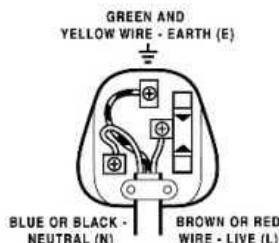
The BROWN wire must be connected to the terminal marked with the letter L
