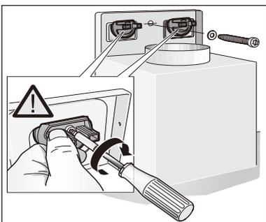
Note: The wall fixings supplied may not be suitable for all wall types, and therefore it is the responsibility of the installer to ensure the wall fixings are appropriate for the surface that the Hood/Flue is being attached to
