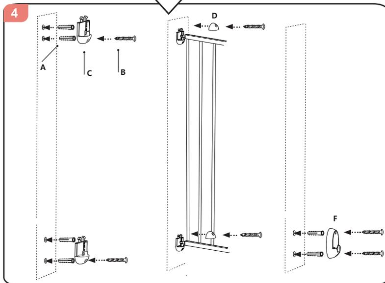
Drill 5 mm hole for the 6 marked positions, then put wall plugs (A), and use screw (B) to fix component (C) and (F).
