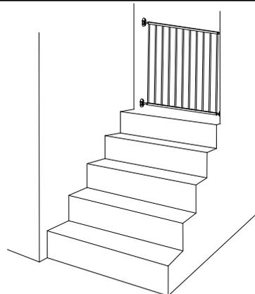
If the safety barrier is used at the top of the stairs, it should not be positioned below the top level.
