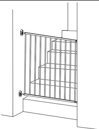
If the safety barrier is used at the bottom of the stairs, it should be positioned at the front of the lowest tread possible.
