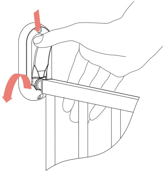
One-handed use, press down the button and lift the gate for two way opening.
