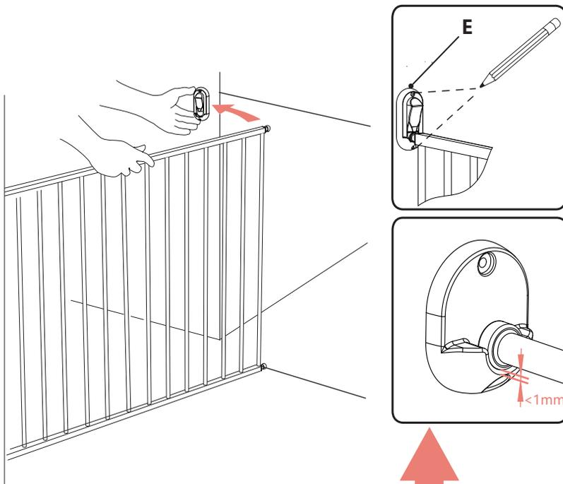
Locate the 2 holes position before (E) to be amounted on the wall.
