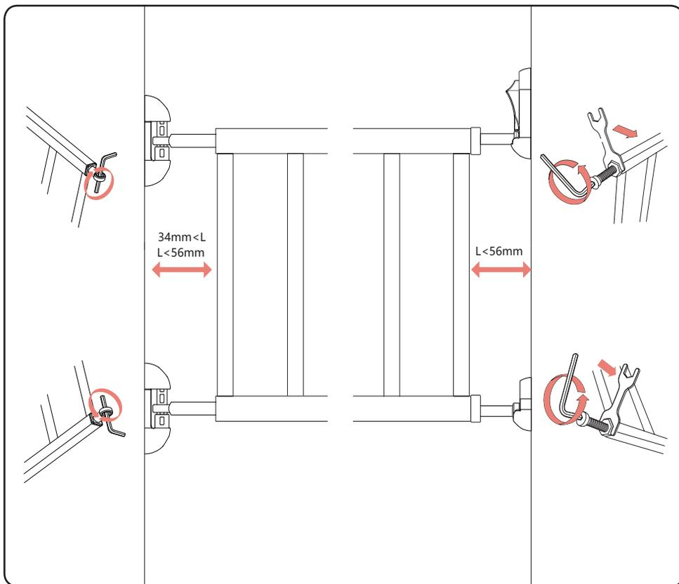
Use the tools provided to adjust bolts (I) and (J) to make the gate width to fit the door properly as below safety requirement:
