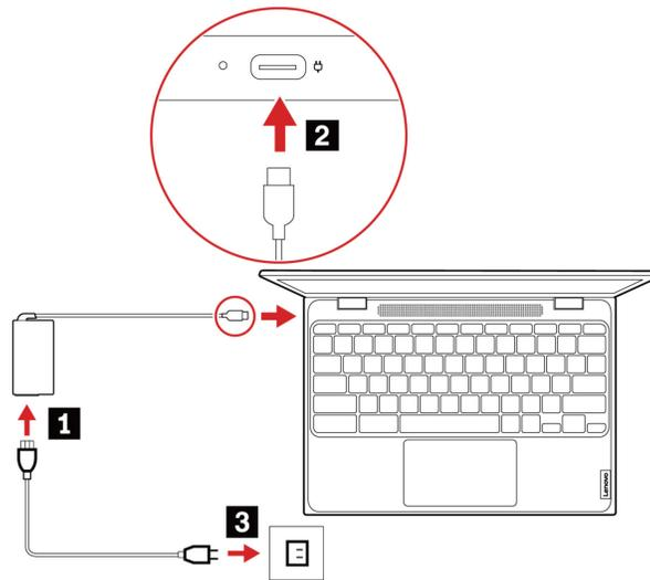
1. Connect the power cord to the ac power adapter.
