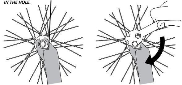
**D** Once the wheel is in place and tight, turn the bike the right way up and squeeze the brake arms together until there is a 1 - 1.5 mm gap between the brake pads and the rim. Both sides should be equal. Whilst holding in place you then need to pull the brake cable tight, and tighten the cable pinch bolt by turning clockwise using the spanner provided as shown.
