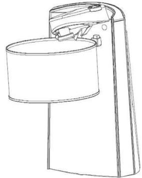
4. Lower the lever firmly so that the cutting blade pierces the lid this will start the can opener working automatically and the can will rotate. It is not necessary to hold the lever or the can during operation.
