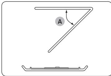
To clean the upper area of the cooking chamber, lower the top heating element by 45° (A) as shown. This will help clean the upper area. When done, reposition the top heating element.
