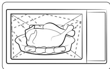
1. The microwaves generated by the magnetron reflected at cavity and are distributed uniformly as the food rotates on the turntable. The food is thus cooked evenly.
