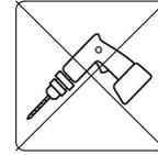
We do not recommend the use of power drill/drivers for inserting screws, as this could
